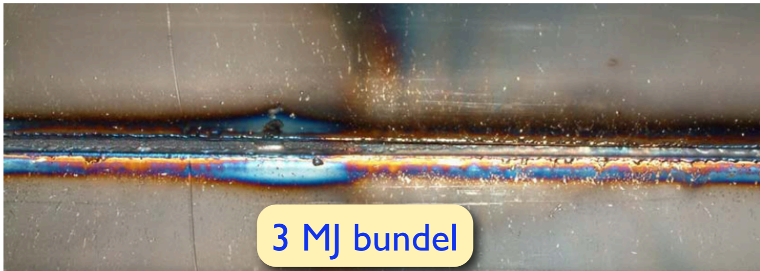
Figure 4. Damage observed on the inside of the vacuum chamber, on the beam impact approximately 110 cm long due to removed material was clearly visible, starting at the entrance.
