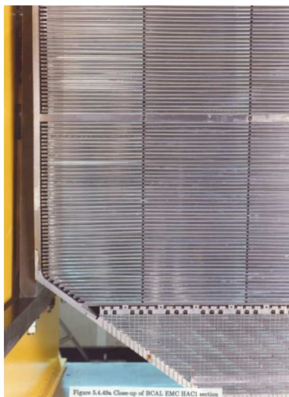
Figure 7.22: Uranium-scintillator structure of the ZEUS calorimeter
